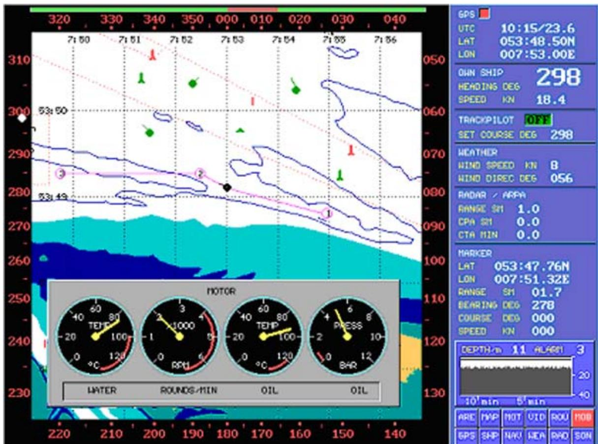
If the motor fails in pressure, temp. etc (too high or too low values) the motor instrumentation will be shown automatically. If you want to control the motor anyhow, you press button 3.
